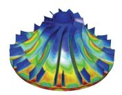
In Pro/ENGINEER Mechanica, we can easily determine where the higher stress areas are on this turbine and make adjustments to the model as needed.
