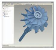
Pro/ENGINEER Mechanica gives you the option of uniformly meshing a model, as we see here, or customizing the mesh for tailored results.
