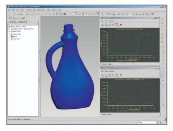
Pro/ENGINEER Behavioral Modeling extension ensures your design meets its requirements. Here we can ensure the bottle will be able to hold the desired mass of liquid.
