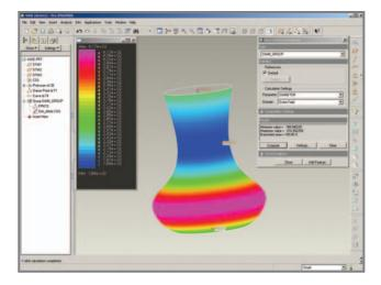
The trial and error approach to get the desired cross-sectional area along a curve can be extremely time-consuming; with Pro/ENGINEER Behavioral Modeling it is fast and easy.
