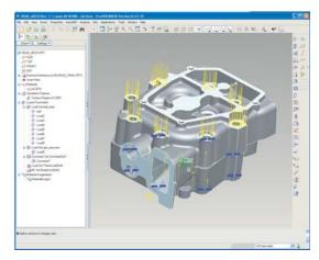
Pro/ENGINEER Advanced Mechanica simulates more accurate real-world conditions for stress analysis by defining bolt preload conditions and internal combustion loads.
